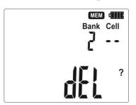
Set the bank number to be deleted according to section 3.2. Set the cell number to • (before 1). The symbol dfl appears which indicates the readiness to delete.
