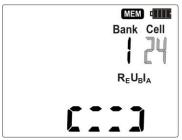
The symbol indicating the content of the cell saved as last, is displayed and after 5 seconds the first result is shown.
