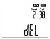
The deletion progress is shown on the display as scrolling cell numbers. When deletion is complete, the meter generates two short beeps and sets the cell number to 1 and the bank number to 0.
