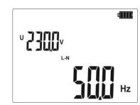
Read the result of measurement: the voltage on the secondary display field, the frequency of the principal.
