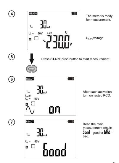
Enter the result into memory by pressing **ENTER**, or see the components of the result of the result of the result of displaying voltage values by pressing **ESC**.
