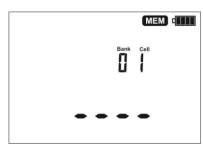
The deletion progress is shown on the display as scrolling bank and cell numbers. When deletion is complete, the meter generates two short beeps and sets the cell number to 1 and the bank number to 0.
